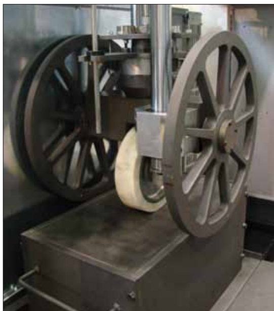
Detailed view of wheel-tracking function of B 120/B26
